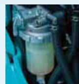
Pre fuel filter with built-in water separator
